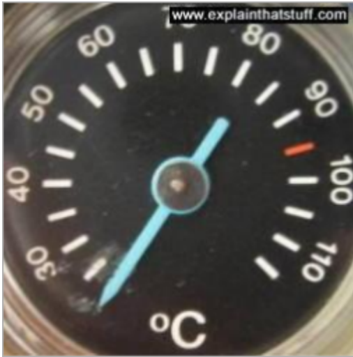
Photo: This dial thermometer shows temperature with a pointer and dial. If you prefer a more subtle definition, it uses its pointer to show a representation (or analogy) of the temperature on the dial.
