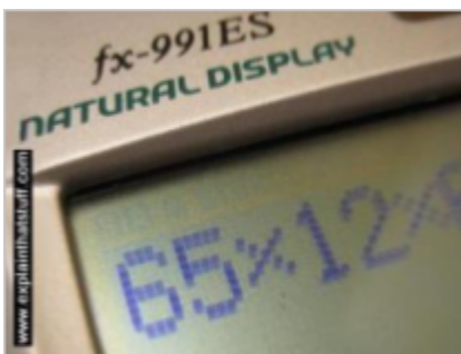
Photo: A small LCD display on a pocket calculator. Most digital devices now use LCD displays like this, which are cheap to manufacture and easy to read.
