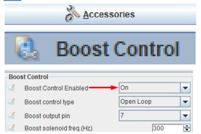
PROTECTION: Enable boost cut to when the value is reached
