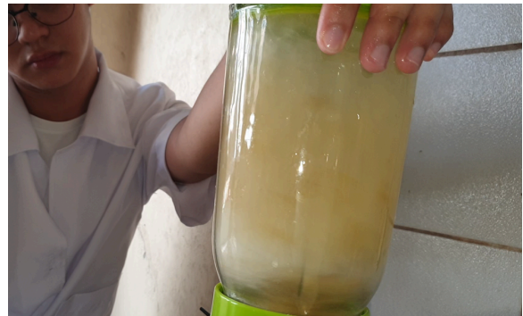
Figure 14 Pulping of cooked husk using blender
