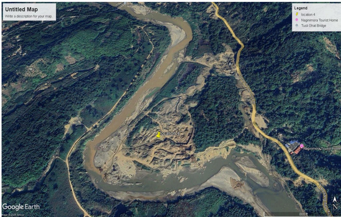
Figure 5b, 2026. Core completely excavated into terraced benches, spoil heaps, a dense haul-road network and working faces cut into the former floodplain terrace. Water in the upstream limb is heavily turbid brown. Bar surfaces markedly enlarged; low-flow channel narrowed and displaced. This frame carries a scale bar (800 ft) and imagery credit (© 2026 Airbus).
