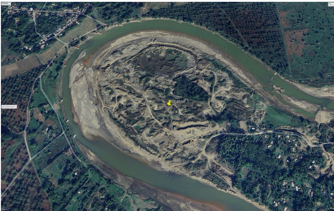
Figure 2b, 2026. Vegetated core effectively eliminated; the interior is stripped to bare substrate and reworked into excavation pits, spoil ridges, benched faces and haul tracks, with standing water in the deeper cuts. Orange-red staining visible on parts of the channel margin.
