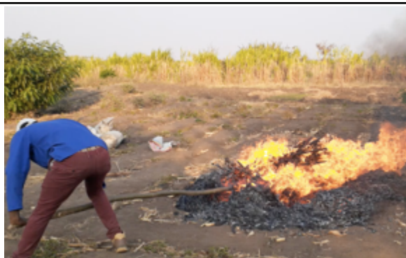
6:37: every time raw biomass is stirred up and starts burning when in contact with the air, the yellow flames revive
