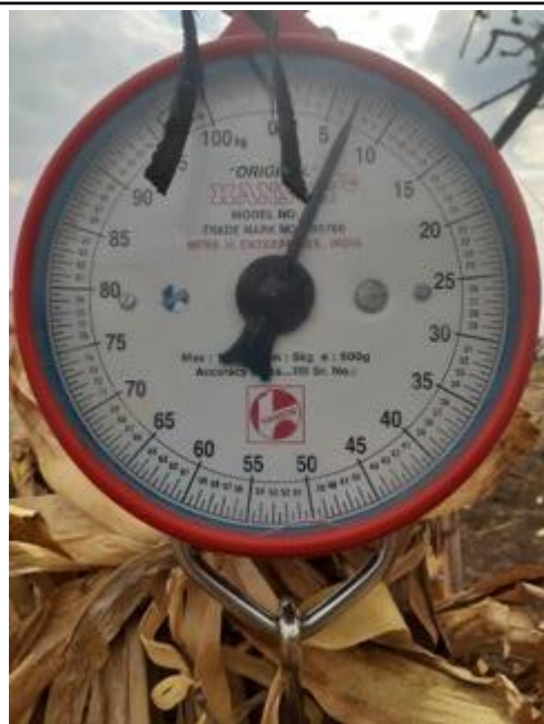
Weighing 100 stalks on a hanging scale = 7 kg The weight of 5 out of 7 bundles was rather consistently between 6.7 and 7 kg.
