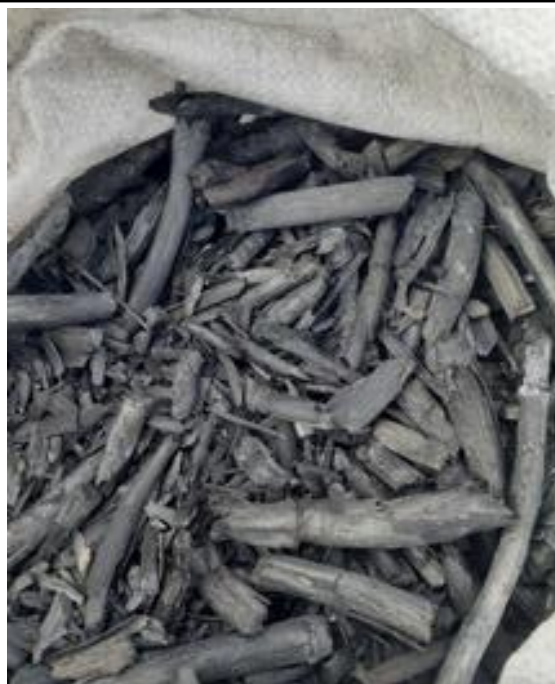
Very good quality char from maize stalks in bag 1: lightweight, brittle, easy to crush to powder
