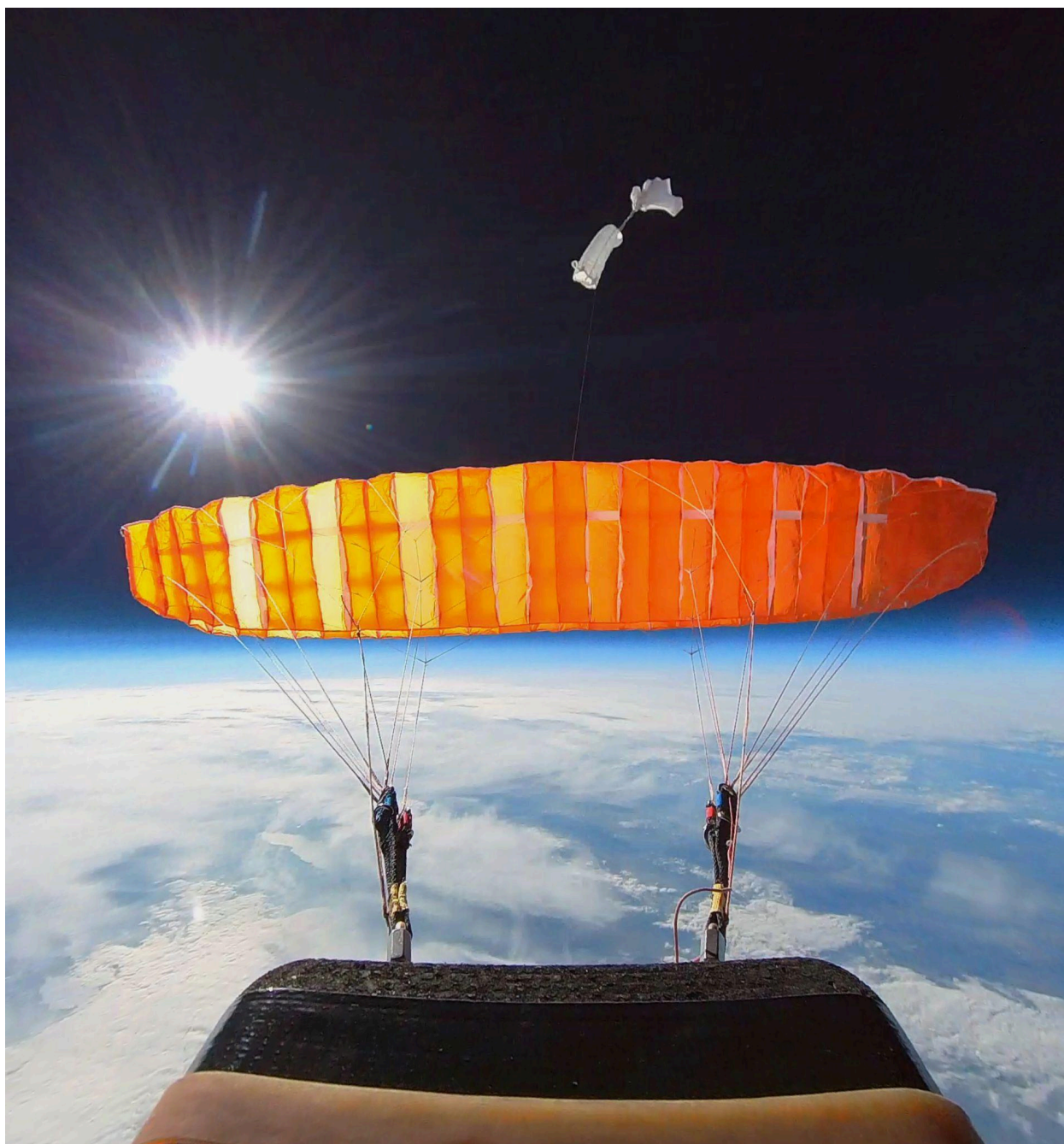
Autonomous robotic glider captures high-res weather and climate data from 0-to-30-kilometer altitude.
