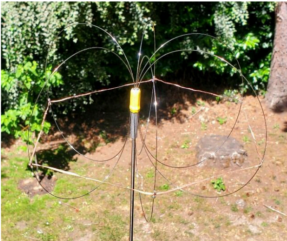
Photo 3 – “Pumpkin” hat with six SS ribs manually inserted into female end of spacer (above yellow shrink tubing). Friction on internal screw threads seize the rib wire mechanically (remarkably well!) and make electrical contact.
