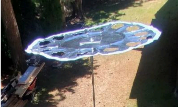
Photo 2 – Solid aluminum disc mounted on top of whip
