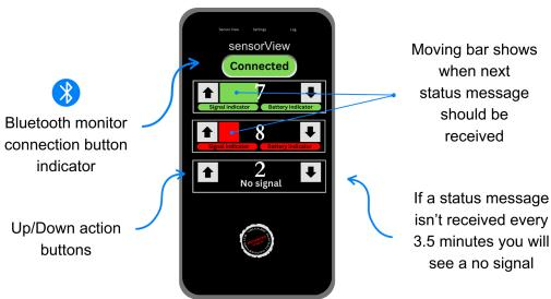
The bluetooth monitor communicates with the barrier arm controllers via the LoRa radio.
