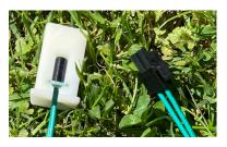
The tilt sensors are inserted into the end of the barrier arms at the hinge point next to the barrier controllers. The sensors indicate whether the barriers arms are up or down at either side of a 45 degree angle.
