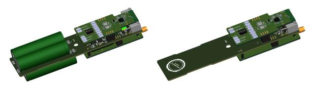
The actView AV494420 (controller) & AV498120 (monitor) are part of a radio control system that allows the remote operation of a linear actuator. The linear actuator moves the barrier arms up and down.
