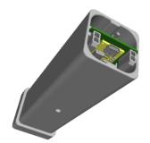
The radio device case protects the radio from the elements and the two are held together by a 6mm pin. It is used in conjunction with the device case bracket which allows it to be mounted in a variety of ways. The radio device case has a metal pad on the top of the case that provides a suitable surface for the magnetic antenna.
