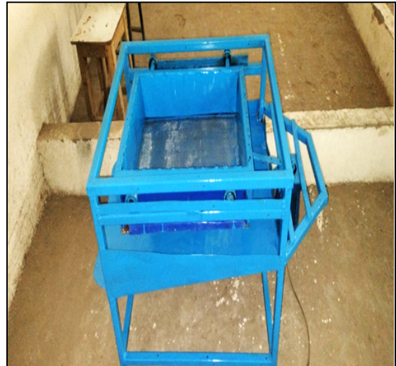
Fig:2 Fabricated image of the Multilayer Sand Filtration Unit
