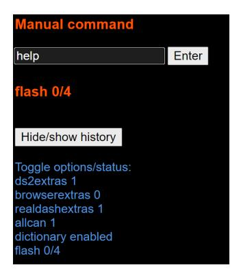
**allcan** lets the DS1 access all the data on the powertrain CAN bus and is generally used together with the other options if you want the DS1 to send extra data to DS2, browser/bTres, RealDash.
