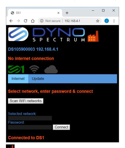
shows that you are connected to the Factory app which the DS1 arrives with. Its job is to connect to the internet and update the OBD app for your vehicle.
