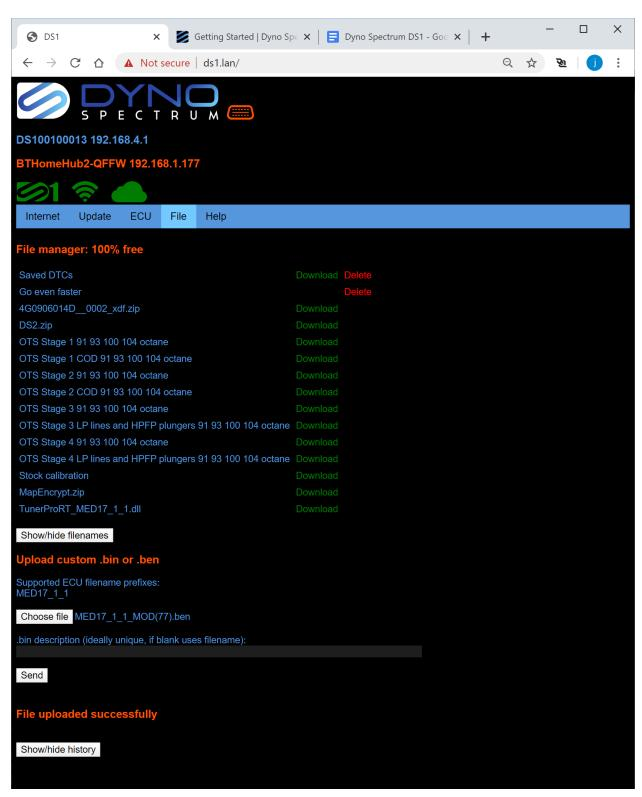
This can be flashed in the usual way from the ECU tab, either Full flash... or Cal flash...
