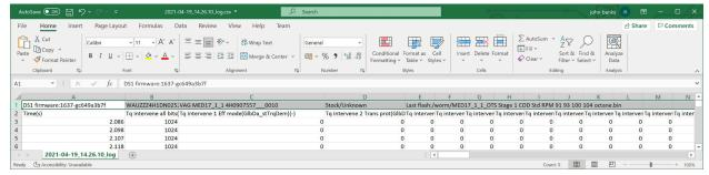
Fix ECU code so that internal log does not get garbage appended when the DS1 is plugged in and then starts its logging. This requires a flash.
