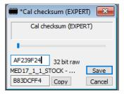
Custom tunes (or people using old OTS maps they want to keep using on 4.0T) need a 4 byte checksum copied from 0x80 (4.0T) to use with the new update. This is because the ECU code has been changed extensively to provide new features. This can now be done using the new "Cal checksum (EXPERT)" item in the Flex Fuel/Map switching folder of the new xdf, also mentioned above. Please ensure that only checksums from matching ECU software version are copied.
