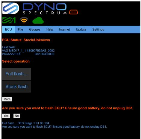
Most will use Full flash... then an OTS map. If you do not click Yes or No within 10 seconds, the question will disappear and the command will be cancelled. **Ignition must be on (dash lit up), engine off. 2019- 2.5T need the hood open to flash** or they will show a "No reply to 31" then "Could not complete ECU command".
