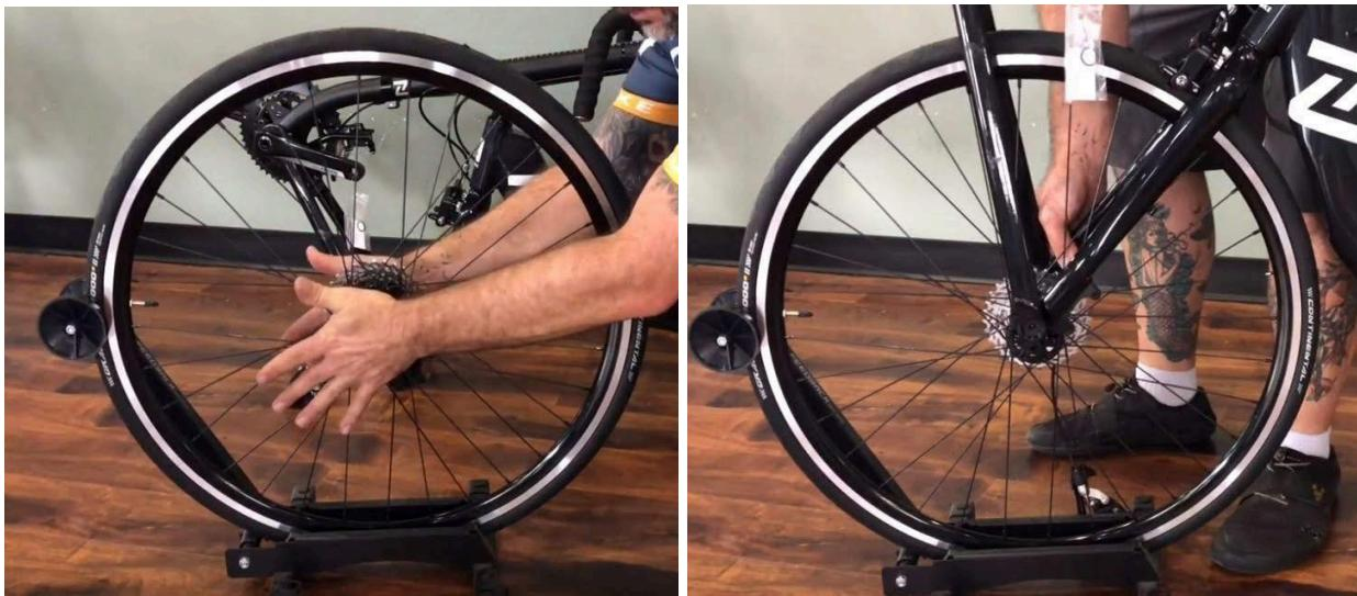
Insert skewer through the front axle with quick release on non-drive side. Note again there are no springs necessary on this skewer. Leave about a finger width of chainstay between the quick release and the chainstay which will leave room to install the derailleur on the other side of the wheel (**image below**).
