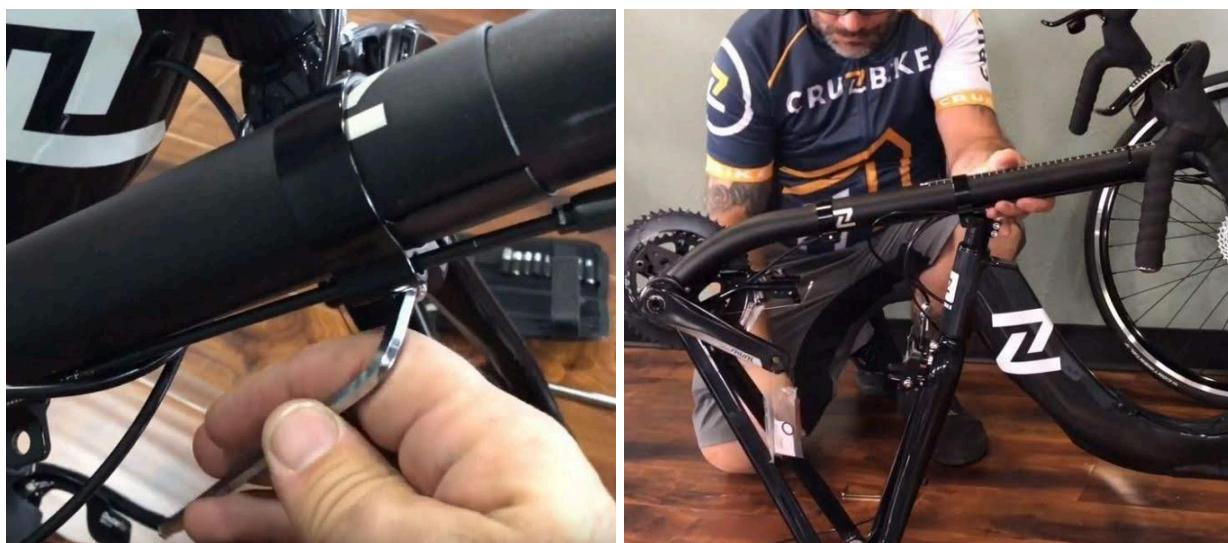
Sit the part of the pivot clamp that is on the slider onto the part of the pivot clamp that is on the steerer tube (**first image below**). Make sure that the middle cable is in the middle between the two parts of the pivot clamp (**second image below**).
