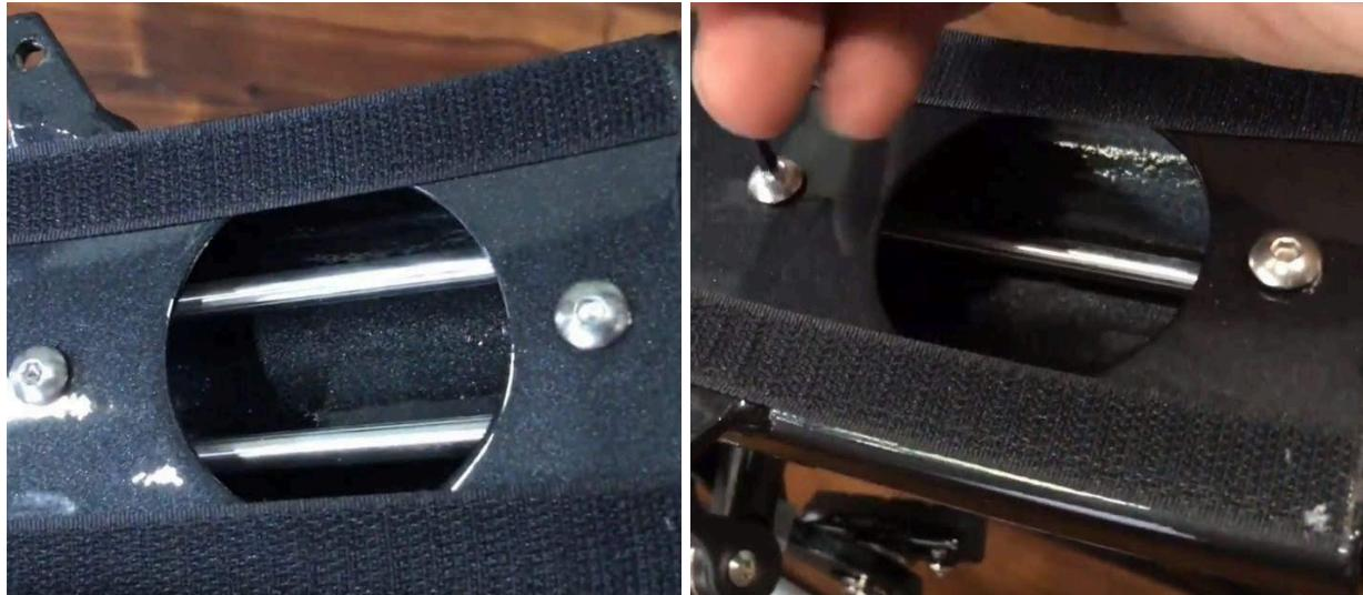
With the Perez Clamp bolts loose, slide the headrest tubes into the frame (**first image below**).
