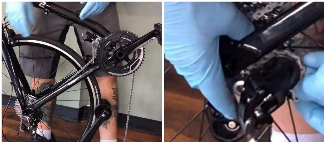
Pull the second smaller jockey wheel toward the front of the bike, then thread the chain underneath the front jockey wheel (**image below**). Make sure the chain links mesh with the wheel teeth. Ensure that the chain does not ride over the metal guard of the cage before wrapping around the furthest jockey wheel.
