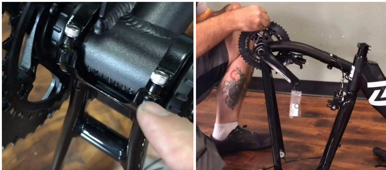
Next, remove the pivot clamp bolt from sleeve (**first image below**). Put two washers on the sleeve side and one washer on the bolt side (**second image below**). It helps to put a little bit of grease or vaseline on the pivot bolt.
