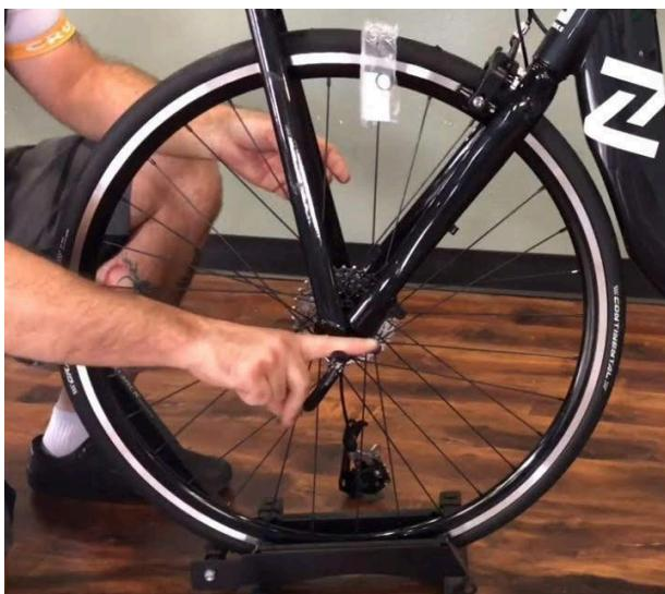
The derailleur hanger has a notched side and a flat side (**first image below**). Slide the derailleur hanger between the chainstay and the fork with the concave side facing in toward the fork (**second image below**).
