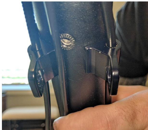
Push the sleeve of the pivot clamp bolt through the pivot clamp making sure the two washers are on the outside (**first image below**). Next, tighten the boom clamp just enough so that it no longer slides from side to side (**second image below**).
