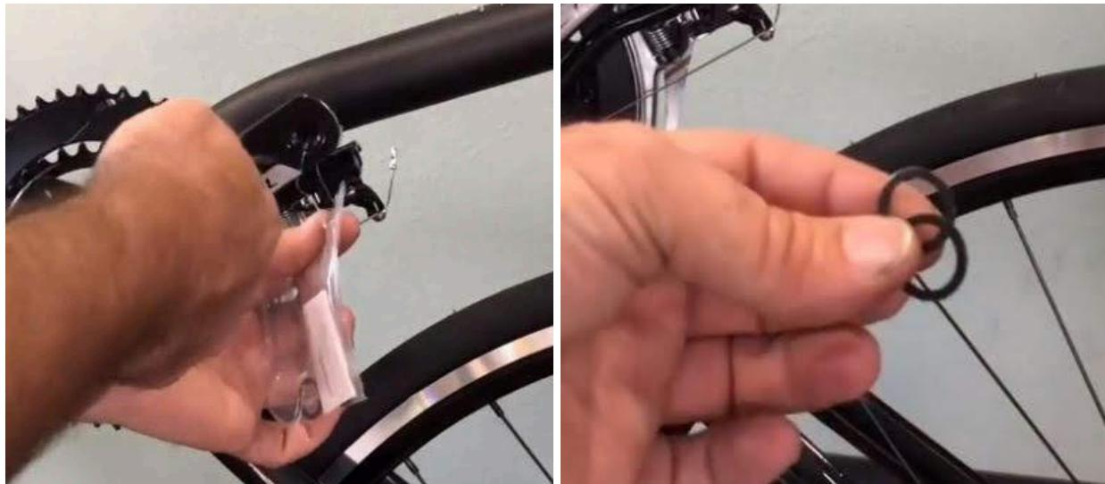
Locate the left and right markings on the pedals inside the pedal mold. Put pedal washer over the end of the pedal (**first image below**) and use 6mm allen built from socket tool, adapter and 6mm bit to install pedals (**second image below**).
