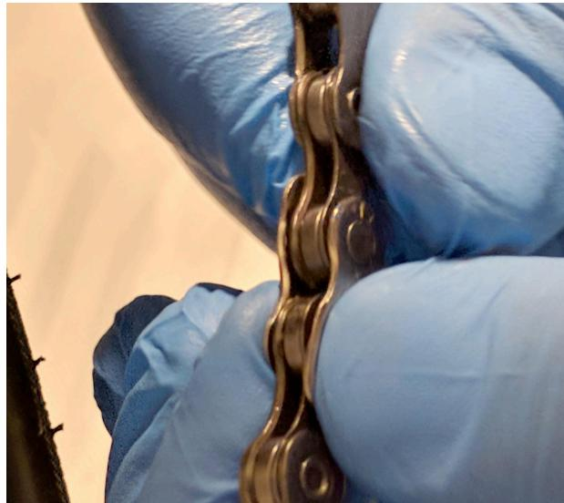
If quick link does not settle into position when pulled (**first image below**) you can place the quick link into the top part of the chain path between the cassette and the front chain ring by very carefully turning the cranks backwards, then push hard on the pedal. That should close the quick link and lock it into place (**second image below**).
