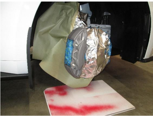
Jacking, Cleaning, Masking, Test Sprays
