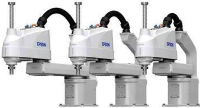
H8 SCARA robots with (from right) arms lengths of 450 mm, 550 mm, and 650 mm
