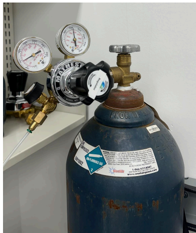
Fig. 8 Needle valve (left), two dials and regulator (middle), cylinder valve (right)
