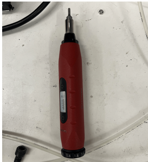
Fig. 12: The red snap-on torque screwdriver. It applies a set torque as it screws dictated by its readout in inch-pounds. There's a dial at the bottom that can be pulled out and spun to adjust the screwdriver's strength.
