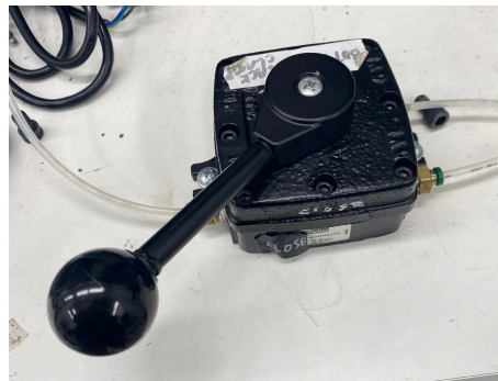
Fig. 9 Left: the switch is in the closed position (see the little piece of black tape on its front face that says “close”). This will ensure pressure is actively holding the clamp together. Right: the switch is in the open position. The clamp will stay closed, unless you press “valve” in the ELLA GUI.
