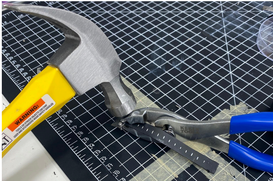
Fig #TODO. Pliers around LMA, hammer positioned in location to hit the pliers.
