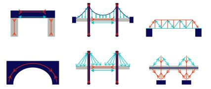
The graphic above shows how different bridge designs can balance these two forces! The more balanced your forces, the stronger your bridge will be.
