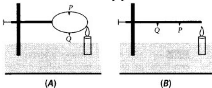
a) Give reason behind falling of pins at different interval.
