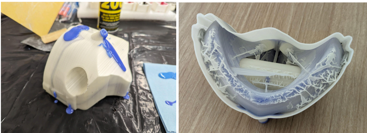
Fig: Mold after Silicone Injection (second Image has bottom layers removed to view interior of mold)
