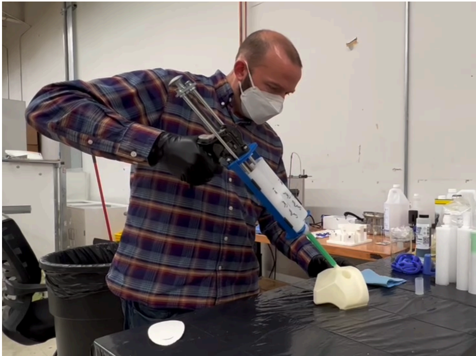
Fig: Injecting Mold with Manual Handheld 1:1 Ratio Dual Cartridge Gun.
