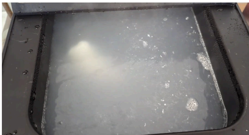
Fig. Heated Water Bath for BVOH Removal
