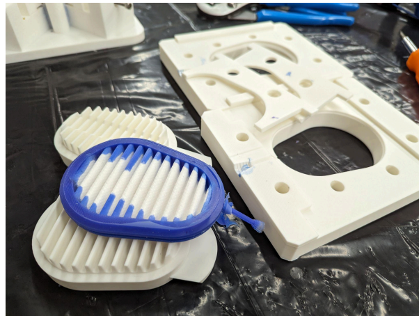
Fig: Filter Mold Disassembly After Injecting Silicone
