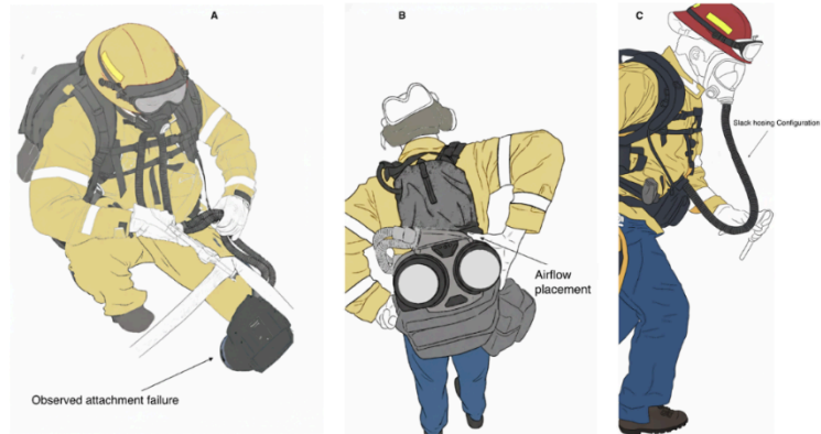
Figure 1. Common integration issues observed during operational field testing. (A) Observed attachment instability, PAPR B. (B) Control placement, PAPR B-D (C) Slack hosing, Configuration B-C.
