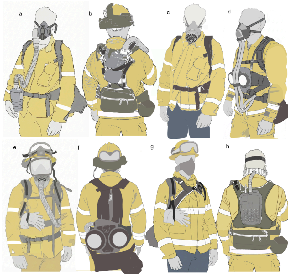
Figure 2: Illustrations of body placement and mounting strategies used across evaluated configurations. (a) Configuration E (front/clip-mounted placement) (b) Configuration E (rear-mounted placement) (c) APR (d) Configuration B-C (front-mounted placement). (e) Configuration B-D (front view; PAPR unit back mounted). (f) Configuration B-C (back-mounted placement) (g) PAPR F, front view (h) PAPR F, back view
