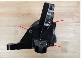
17. Install the supplied brake caliper mounting bracket onto the upright using the supplied M12 x 25mm bolts. If your caliper bracket uses a countersunk bolt you will not use washers underneath the head of the bolt. Torque the caliper bracket bolts to 85 ft lbs using a blue thread locker on the threads.
