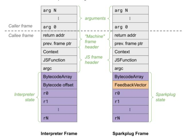
The one difference is that it overwrites the bytecode offset slot (which is not needed) with a cached feedback vector.
