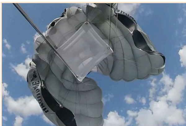
RDS rings positioned on the trailing edge of this fine mesh slider act as the 5th and 6th grommets.
