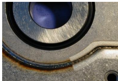
b Metal surface oxide laser cleaning
