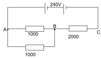
Determine the potential difference between A and B
