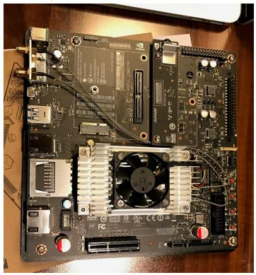
The TX1 is actually an SOM (System On Module) about the size of a credit card (though a bit thicker). The heatsink on top dissipates heat and the whole thing is attached to a carrier board with four screws and a special connector.
