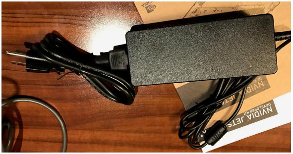
Please note that the power brick outputs 19V. This power brick produces a voltage that is incompatible with the TK1 boards. If you plug this into your TK1 board then bad things will happen. The TX1 can run off of 12V but please make sure that your polarity is correct before plugging it into another power source.
