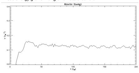
Excitation of (5,6) mode, with frequency around 67kHz
