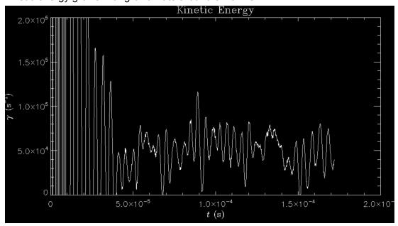
Excitation of (6,8) mode, with frequency around 69.5kHz
