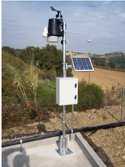
Fig. A2.5.3 Conventional weather station that measures various parameters, including precipitation
