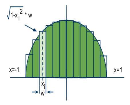
This diagram shows 12 rectangles of equal width w that approximately cover the green semicircular area. Each rectangle is positioned over a subinterval of the x-axis interval [-1,1], and the height of a rectangle is the function's value at some value  $x_i$  in that rectangle's
