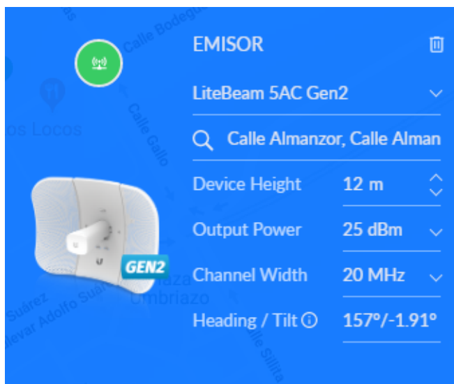
Antena Emisora: LightBeam 5AC Gen2
