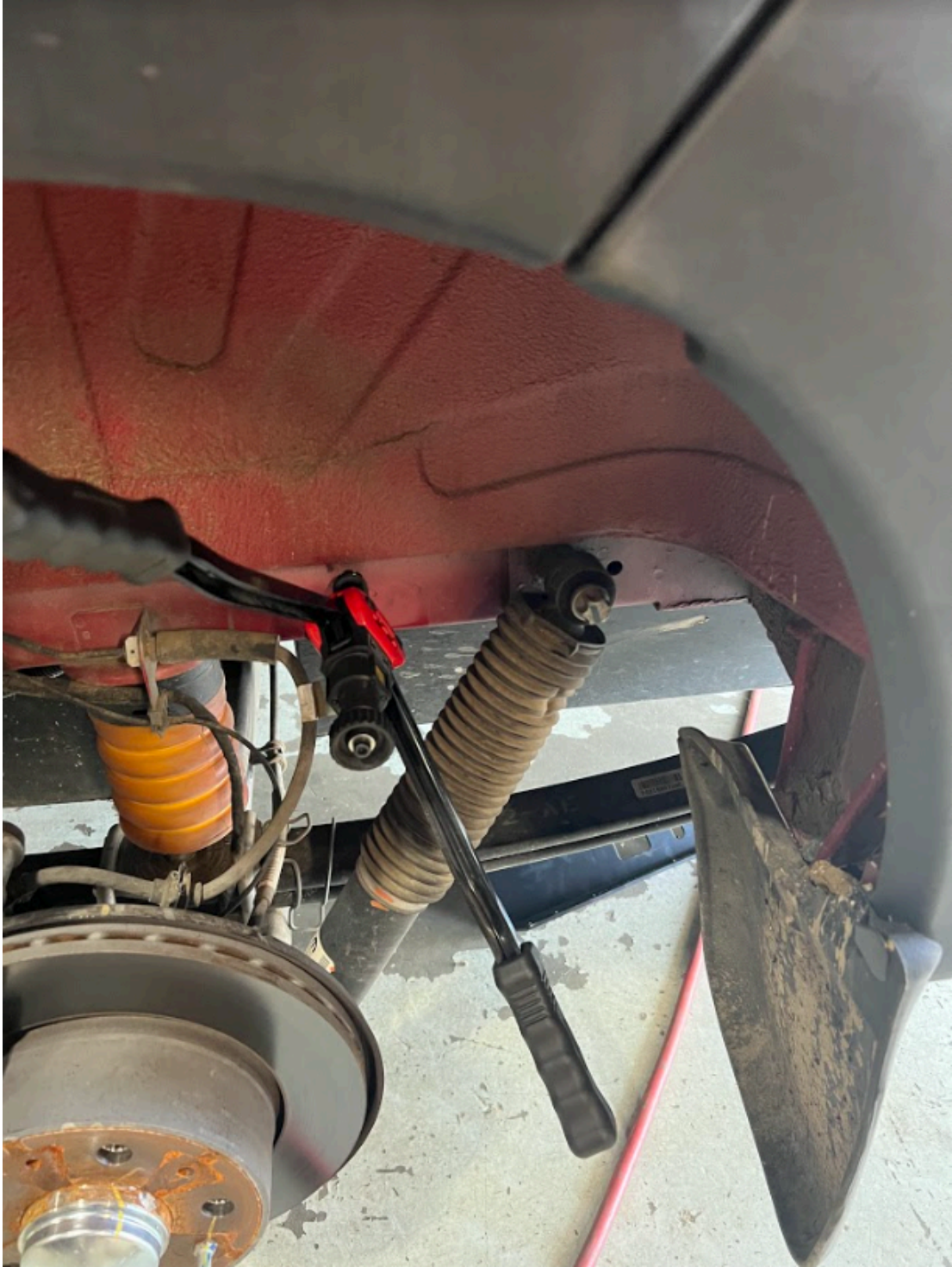
Once Nutsert install is complete it should look like photo below.
