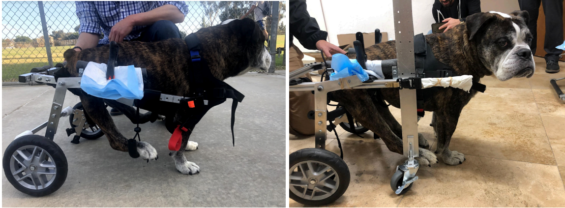
Figure 22. Before (left) and after (right) prototype testing on the adjustable 80/20 frame.
