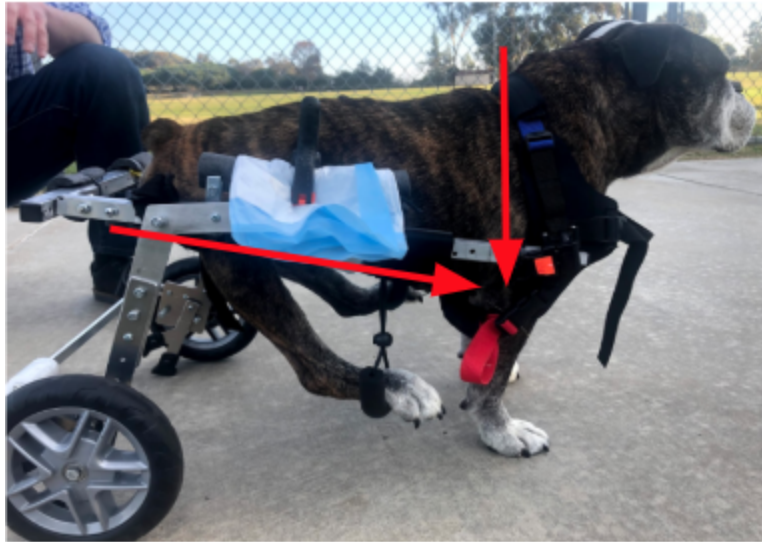
Figure 7. Previous 156B team's folding, rear-support wheelchair.
