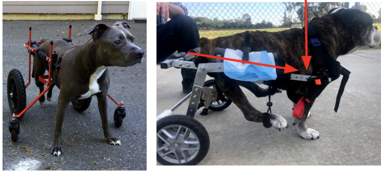
(Left) K9 Carts. Industry rear-support wheelchair features 4-wheels. (Right) Previous model of Bodie's wheelchair rests front frame on shoulder harness.
