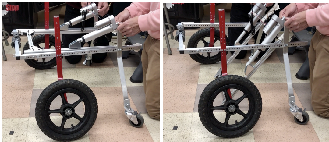
Figure 15. Linear actuated system in up (left) and down (right) positions.
