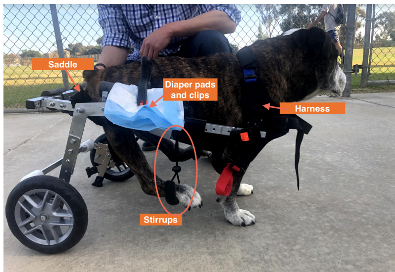
Figure 10. Comfort components that are in contact with Bodie's body.
