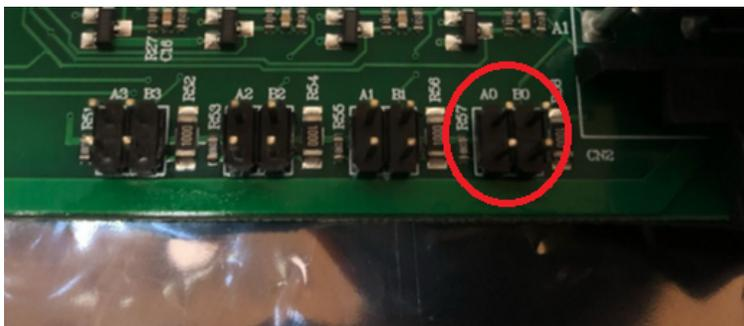
The second pictured example below, channel 0 has been set to add an additional 1,000 ohms resistance in parallel. Channel 2 has been set to add an additional 100 ohms resistance in parallel.
