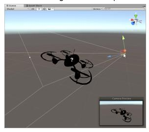
**6)** If your drone has propellers; drag them into the Propeller Array on the PA\_DroneController(script) this will make them spin around the Z Axis.
