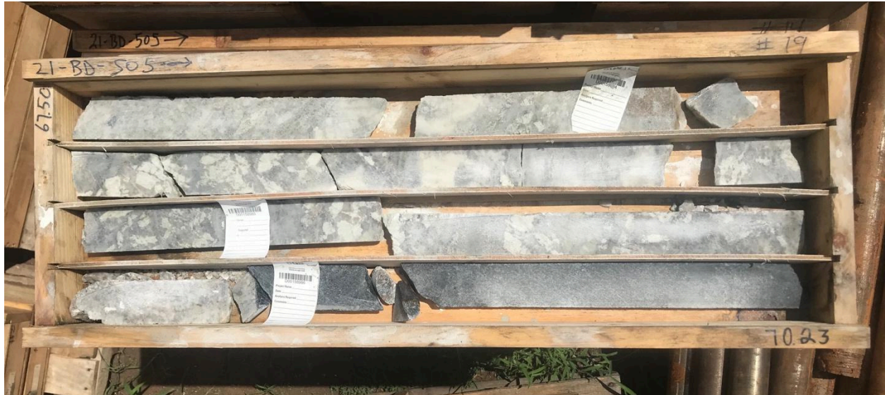
Figure 9 is a photograph of box #19 of hole 21-BD-505 after it has been cut, sample and archived. The Spodumene pegmatite was sampled as well as a 1m shoulder (buffer) above and below the pegmatite interval. The sampled core is half core. One half of the core is put back in the box to serve as permanent record of the drill hole. The other half is bagged and sent to a geochemical testing and certification company for 4-acid digestion ICP-OES analysis. This analysis is very similar to the analysis required for soils, but OES has a higher detection limit for multi-element analysis. The analysis can be customized for a specific deposit to test for specific mineral suites. In the early stages of a project ICP-MS is more practical as it is more accurate although more expensive. For precious metals, the most accurate form of ICP analysis is finished by fire. Often, multiple finishes can be done for the same sample for QA/QC. This is done in high grade zones by duplicating the sample. The samples can also be duplicated by quarter core samples, where the core is cut in half, then the sampled half core is cut in half producing a quarter core cut sample. The two quarters are divided into 2 separate samples which should produce nearly identical ICP results. If the duplicate samples show different results, it could be due to issues in the test processing or potential nugget effect of the material in question.
