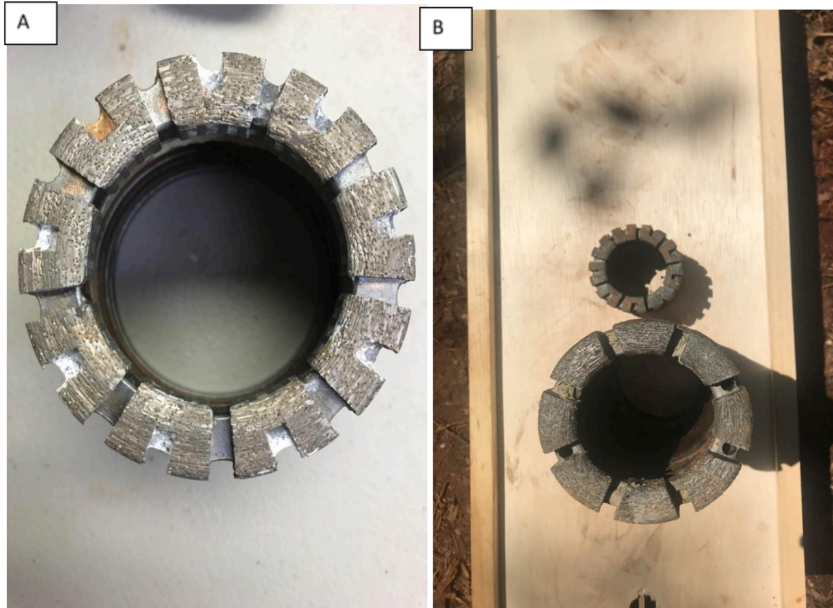
Figure 5 a-b are photographs of diamond core drill bits. These bits have small sand sized industrial diamonds evenly distributed through the steel tooth matrix. The combination of hundreds of these industrial diamonds working in tandem allow the drill bit to cut through the rock with general ease. This process allows the drill string (combination of bit and core rods) to slowly lower down into the rock capturing the cylindrical shape of diamond drill core within the core barrel. The grooves going around the bit function as water or “drill mud” vents. These allow the water or drill mud to flow between the teeth as a cooling medium as well as a lubricant for the rest of the drill string. As the drill mud cools the teeth of the drill bit, this allows the steel diamond matrix to stay cool rather than melt which would in turn release the cutting diamond teeth. This cooling allows the drill bit to last significantly longer when compared to an uncooled bit. Over time, the diamond teeth wear down, the steel is sheared or melted away and new diamond teeth are exposed further self-sharpening the bit. Figure 5 a is a nq sized diamond core drill bit which is better for drilling competent rock at depth. Figure 5 b is a hq drill bit next to an nq drill bit. The hq is a larger bit with a greater diameter and is suitable for drilling less competent rock. Often a larger core size bit is used to drill through less competent overburden/saprolite. Once the drill is a few runs into bedrock, the driller will reduce the drill bit size and set casing around the drill string in the ground to reduce the risk of clays swelling and stabilizing the hole from collapse. Smaller diameter drill bits are used at depth due to lower cost of parts and materials, less drill mud and water required, and faster drilling due to less material to remove. The combination of these decrease overall operating costs if nq core can be used.
