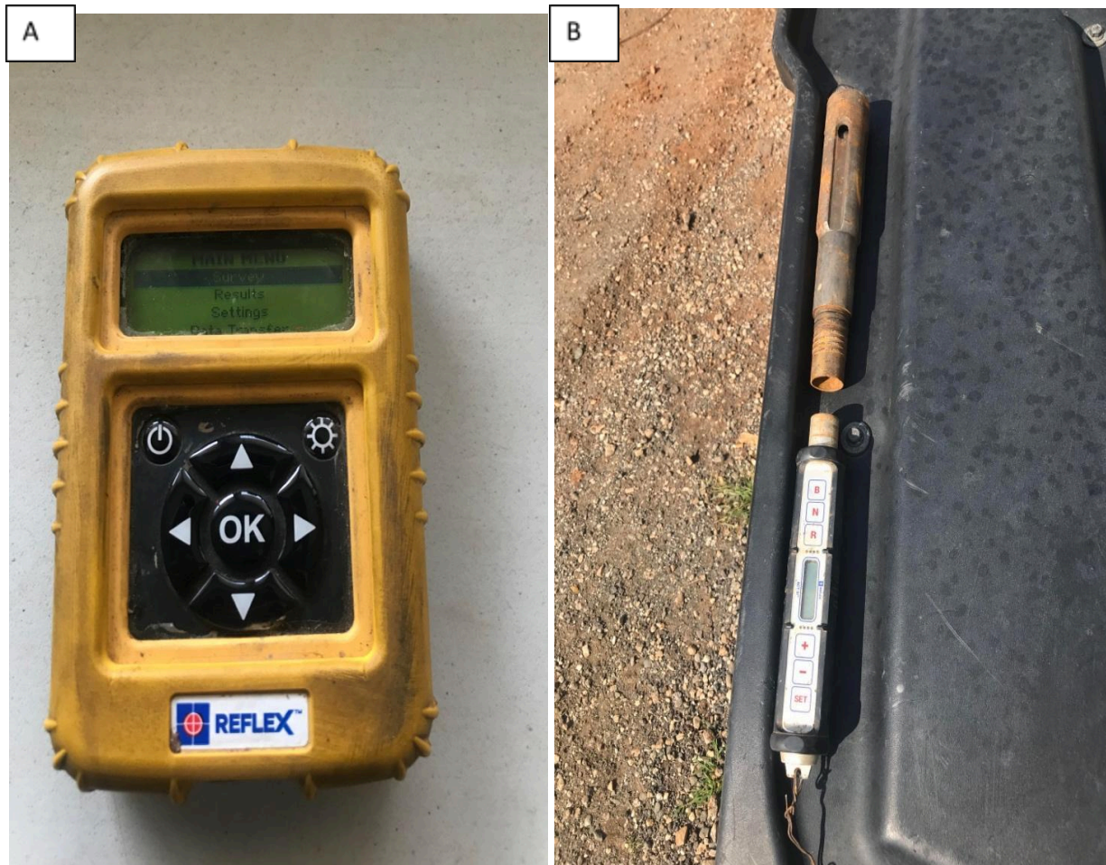
Figure 6 a-b are photographs of down hole testing tools. Figure 6 a is a down hole survey pad. The survey pad is used down hole to define the orientation of the drill trace. The survey pad measures and plots the 3D path of the drill trace. The tool works by magnetic sensors or gyroscopic sensors. The survey pad in figure 6 a works sending a magnetic reading down hole and noting the azimuth and dip along the drill trace. In a system that does not have an abundance of magnetic material, the magnetic survey is more cost efficient. If there is an abundance of magnetic material, the north-seeking Gyroscopic (N-seeking gyro) sensors are best, as they will not be disturbed by the magnetic field. Figure 6 b is an orientation tool which is used determine the “up” direction of the drill core. Down hole, there is a core barrel extender (top) that defines the “up” by an optical sensor down hole that notes the degree of rotation as the drill spins. When the run is brought up to surface, the orientation remote (bottom) is inserted into the core barrel extender extension. Then the orientation remote gives a reading of “OKAY”, or a set of arrows denoting a clockwise or counterclockwise rotation to align the cores “up” direction with the up direction reading of the rod extension. Once the core is in line with the “up” direction, it is leveled and marked going along the cores “up” direction.
