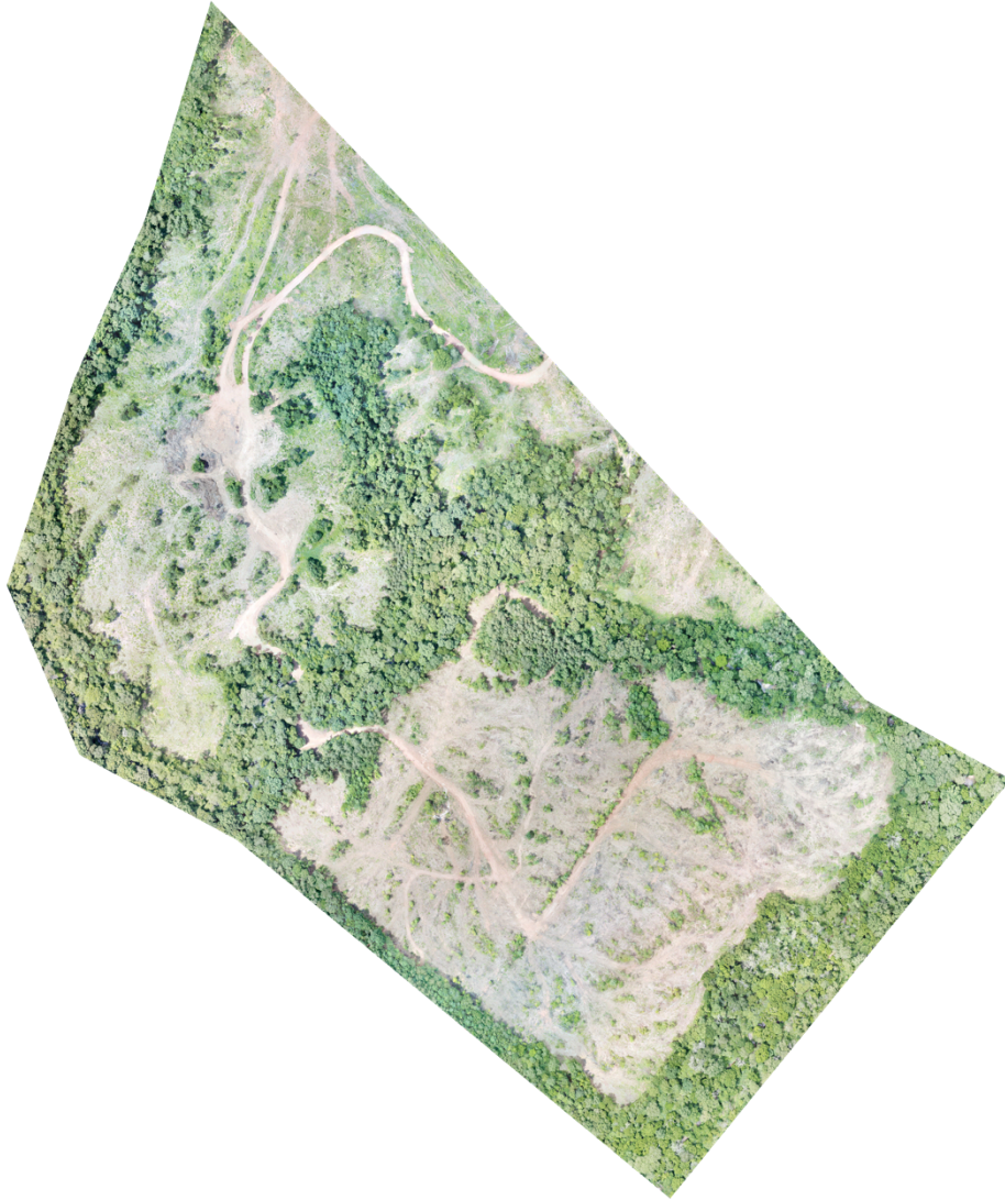
Figure 3 is an orthophoto with 1.6-inch resolution taken from a DJI-Mavic Pro drone with the aid of Drone Deploy flight programming and processing software. The official drone deploy orthophoto report can be found here . This orthophoto was used for multiple purposes including supplementing field mapping as well as high accuracy topographic surface studies for water flow and mine engineering plans. There was an autonomous flight plan developed in Drone Deploy to create this orthophoto. The flight plan captured roughly 1000 pictures with 80% overlap (both front/back and side/side overlap of 80%) producing this orthophoto with a 1.6-inch resolution. Each image is taken with a recorded GPS point, camera azimuth, camera inclination, and GPS accuracy (X,Y,Z). There are external attachments that allow enhanced capabilities of the drone such as lidar, multispectral and hyperspectral imaging.
