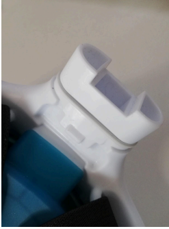
Figure 5: Easybreath V1 connector with rubber ring. The center channel is for inhalation, the two outer channels for exhalation
