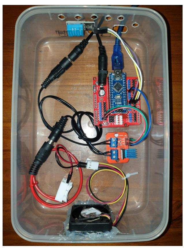
• Top (blue module): DHT Temperature/Humidity Sensor
