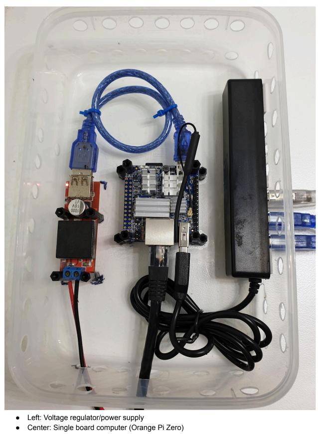
• Right: 6 port USB hub allowing up to 6 devices to be connected
