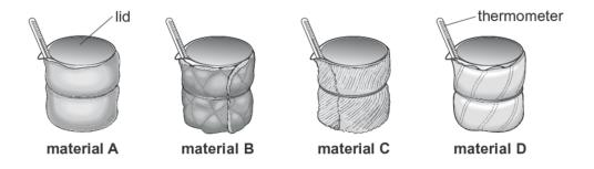
They wrapped each beaker in a different material, then recorded the temperature at the start and 20 minutes later.
