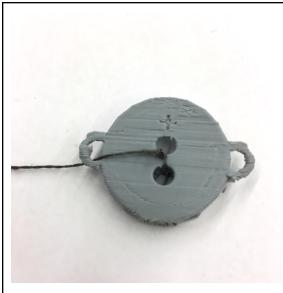
Tie one piece of conductive thread through the holes on the POSITIVE side of the battery holder and loop it through a hole on the side.
