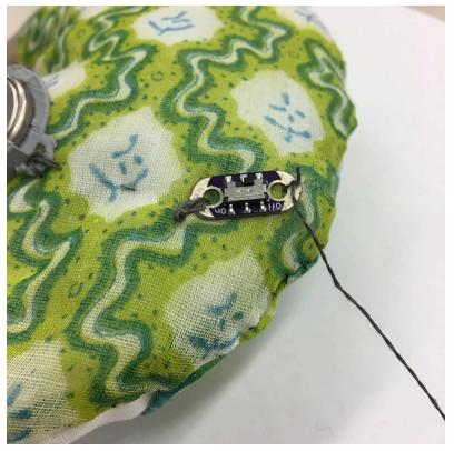
Cut the thread and tie off the switch at each hole.
