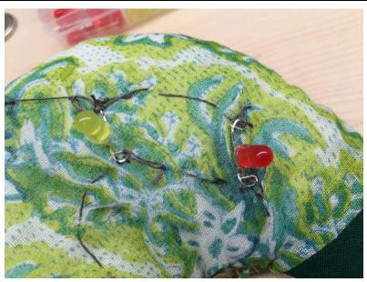
Here is how I sewed my LEDs. When you get to each curled leg, loop through a few times to fasten it well.
