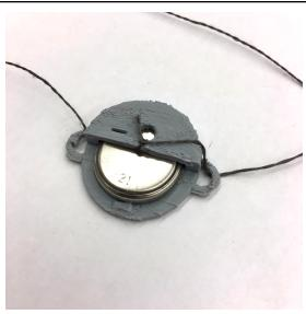
Tie a **second** piece of thread through the hole in the NEGATIVE side of the holder and loop it through the hole in the other side. Slip the battery into the holder with the FLAT SIDE DOWN so the positive and negative charges travel in the right directions.
