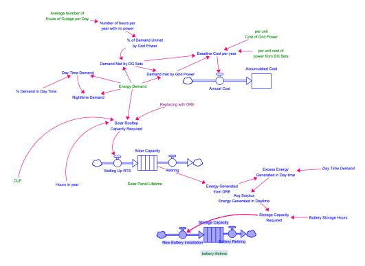
The cost of the DRE system is computed using the capex and opex of the solar rooftop system. Capex times the new installation gives the capital cost and the opex times the online capacity gives the opex per year. These accrue in a stock of total accumulated cost over time to give the cumulative cost. The battery capex is also accounted for, at the time of installation and then every time the battery is replaced (according to its lifetime).
