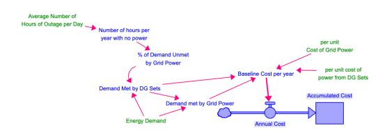
In a scenario where we replace the energy supply with a DRE system in the form of a solar rooftop-battery system, the model aims to meet the entire demand through 100% DRE. It first computes the capacity of solar rooftop required in order to meet all of the demand. This is computed using the expected CUF of solar (A user input) and the demand to be serviced .
