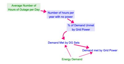
The cost of power in the baseline case is determined using the units of power serviced by the grid and by the DG set and the respective costs per unit of each, all specified by the user. This gives the annual costs, which also accrues in a stock of accumulated cost, giving the cumulative cost of power over the years.
