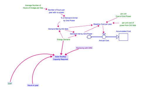
The model then installs the required capacity of solar panels in order to meet the demand. This capacity comes online and stays online as the stock of total onboard solar capacity for its lifetime (Lifetime is also a user input).
