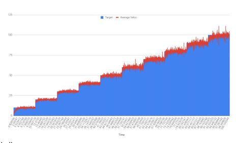
One test with ramping enabled. The red line is the average velocity of all the motors, and the blue is the target velocity.
