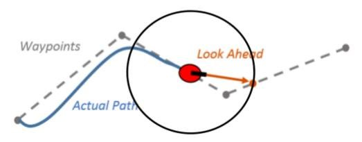
In order to do pure pursuit, other controls are needed, and these include: field centric driving, field centric odometry, PID (Proportional Integral Derivative), and we also used feed forward.
