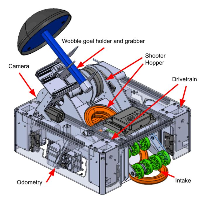
Our robot consists of **FIVE** main parts. There is the wobble goal holder and grabber; the intake and conveyor; the shooter, indexer, and hopper; the drivetrain; and the odometry pods. All of these parts are connected to a central REV control hub and expansion hub. We use a REV battery to power our robot.
