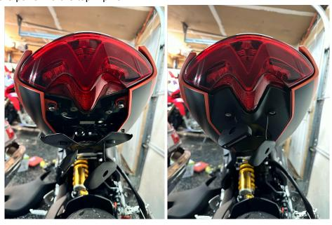
8. Install 2 of the supplied H4 screws and washers into the signals, while making sure to not kink the wires during mounting. Make sure the turn signals are rotated to be as rear facing as they can be without stressing the plastics. They should sit flush as shown in the image below. Feed the wire and rubber grommet into the opening between the bottom mounting points. Install the remaining 2 H4 screws for the plate mount.
