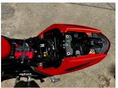
3. Unplug fender harness via connector shown.
