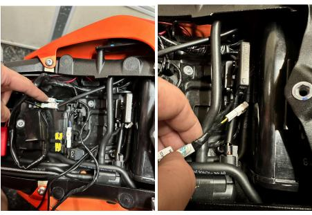
10. Using zip ties, secure the extra parts of the harness and the turn signal wires. (you may not have as much extra wire as shown)
