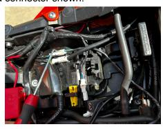
4. Remove the 4 T30 bolts from the underside of the tail and pull the connector through the rubber grommet. Disassemble the fender and remove the harness from the tail.
