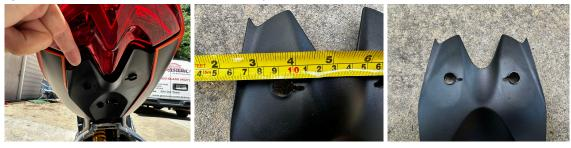
7. Feed the turn signals through the holes and route the wires through the opening towards the front, going around the outside of the bottom mounting points. While holding wires back with one hand, push the beveled pin into the subframe so the panel is slightly hanging. This will make it easier to work with. Pull the wires all the way through and secure the panel via the top 2 pins.
