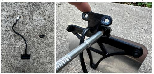
6. Pull down on the underside panel from the top to remove it. Measure out 7mm from the edge of the hole and drill, using a 7/64 drill bit, through the panel for our turn signal wires. Use a pair of cutters or utility knife to connect the two holes.
