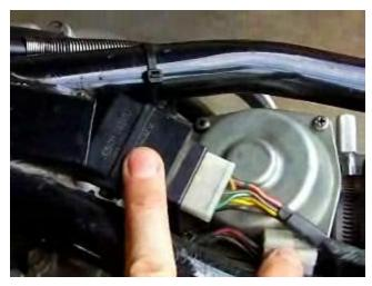
Try to run the wiring harness below the frame rails to avoid clearance issues with the tank. Zip ties are very useful for keeping things organized. (The white connector shown on the left connects to the indicator light assembly of the tank panel):
