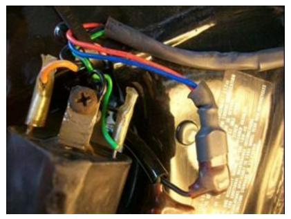
The connectors of the rectifier can be routed through the hole in the top of the battery box. The velcro strap included in the kit can be used to secure the battery:
