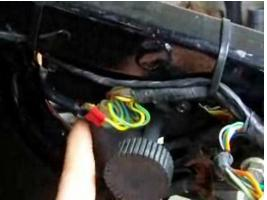
Extend the keyswitch wiring. Cut the connections to the stock keyswitch and splice in longer sections of wire. The exact length depends on how you choose to run the wiring harness, but approximately 24" should suffice. You can use solder and heat shrink for a clean appearance:
