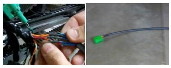
Note: You can extend the wiring on the keyswitch end or the wiring harness end. Just make sure the wires attach to the connector in the same positions. Labeling the wires and taking a few photos is helpful before you make any cuts.
