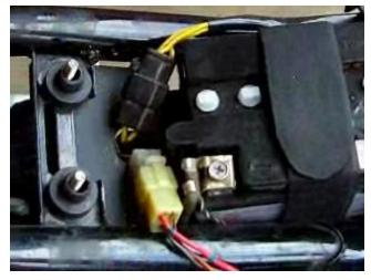
The large relay shown below to the left can be mounted in it's original location above the carb. The decompression solenoid connector (right) is not used:
