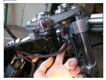
In the photo below, you see the red wire of the gauges and the blue wire of the tachometer tied together and connected to the horn wire with a female flat style connector. The green wire of the tachometer is connected to the negative terminal of the ignition coil. The black wire of the gauges is grounded to the ignition coil screw:
