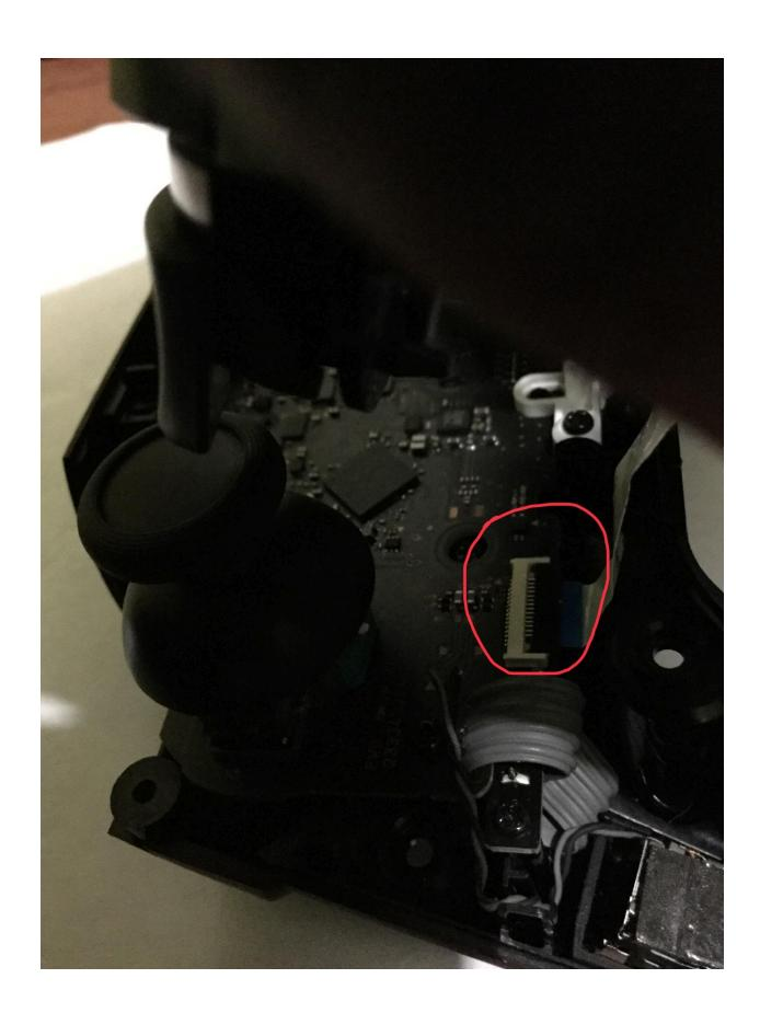
Inside the Pro Controller, you will see that the ribbon cable is attached to a flap that connects it to the motherboard. You can simply lift up the flap that is circled red to disconnect the ribbon cable and put aside the top part of the Pro Controller.
