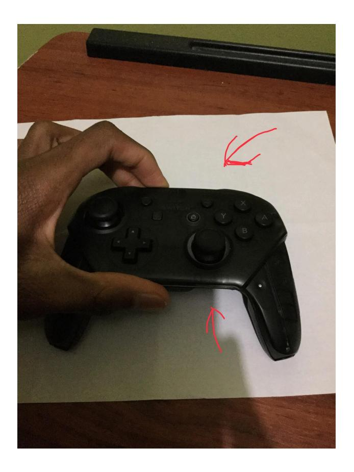
Now gently but firmly, use both hands to take apart the Pro Controller. Be extremely cautious, because there is a ribbon cable right below that be damaged if it is strained but simply opening it up won't do anything to it. If it is damaged or the connection to the controller is loose, it can have adverse effects such as not registering button inputs, gyro controls not working and NFC capabilities not working.
