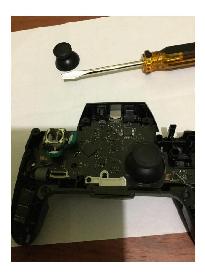
Take your Flathead Driver to very carefully, pry open the sensors. Do not use too much force to do this. Once you have them open, take your tweezers to remove the Analog Stick Sensor Wheels and discard them. Optionally but very recommended, you should be using rubbing alcohol to rub along the sensor just for good measure.
