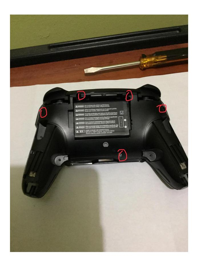
Place back on the back part with the **Nintendo** logo branding on it, be sure to snap the top and bottom parts of it snugly into place, then rescrew the four silver **Back Screws**.
