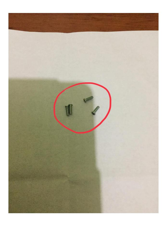
Take off the back shell with the **Nintendo Logo** on it, and you will see the battery along with five short stubby screws that you will need to remove that I will call **Entry Screws**. Remove the battery then unscrew all five Entry Screws.
