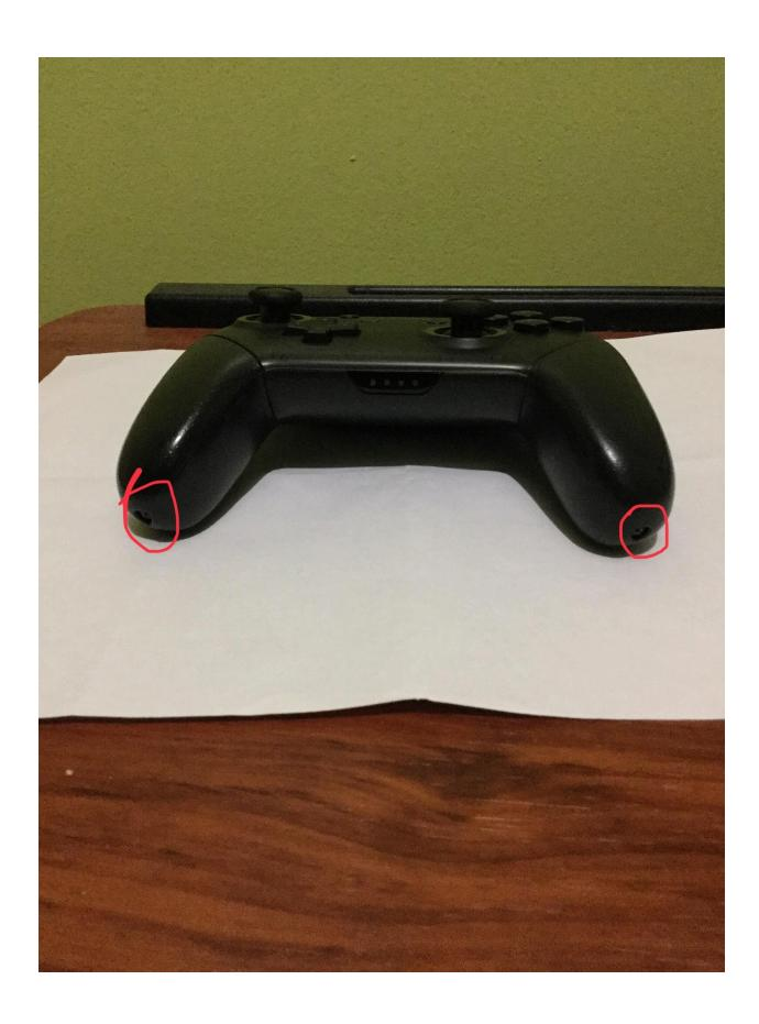
In order to enter your Pro Controller, firstly you will need to take your #0 Phillips Head Screwdriver and unscrew the two screws that are under the grips, then slide off the grips. These two screws I will be referring to as **Grip Screws**. They are small so keep them somewhere safe.
