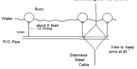
It is important to replace missing buoys. Using the course with missing buoys can damage your boat and the course. Your prop can hit the stainless steel cable or the PVC pipe.
