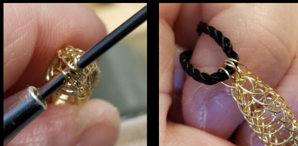
Image 3: Aligning loops to allow for cord. Image 4: Cord inserted through aligned loops.
