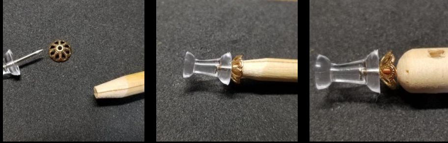
I sharpened the end of one dowel to allow for easier access and added a coil to the other to accomplish the same thing.
