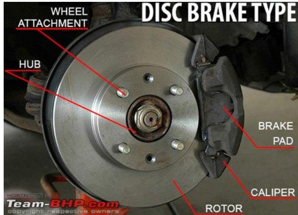
Figure 1: How Calipers and Brake Pads are Attached (3.C)
