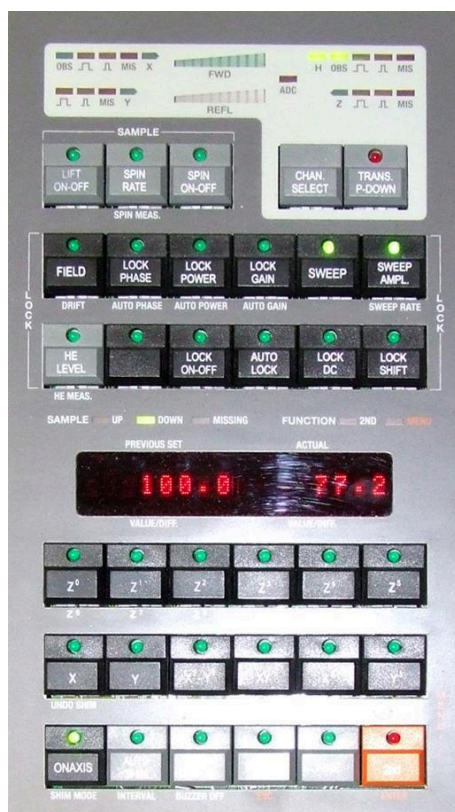
Figure 19. The control panel for sample handling and magnet control as seen from above
