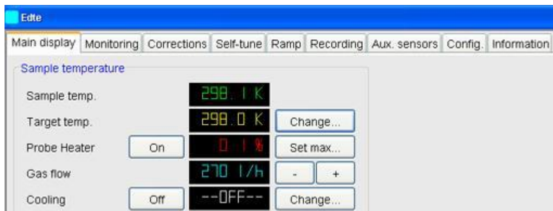
Figure 38. The Main display tab of the edte window for temperature control
