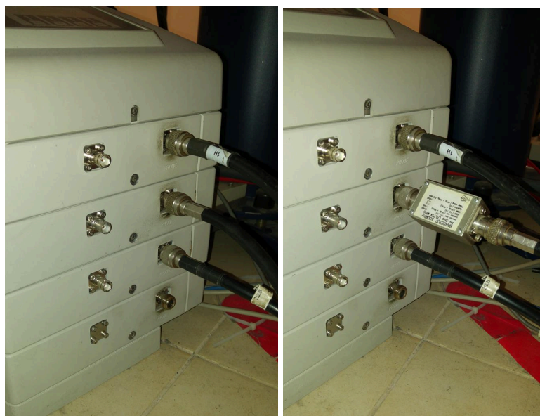
Figure 10. Connections exiting the preamplifiers at the front for regular acquisition. The deuterium stop filter on the broadband channel (2nd from top) is optional and has no effect on regular ^1\text{H} acquisition.
