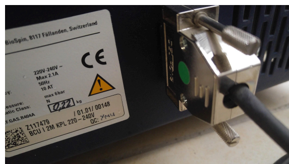
Figure 8. Signal cable connected behind the BCU1 cooling unit.
