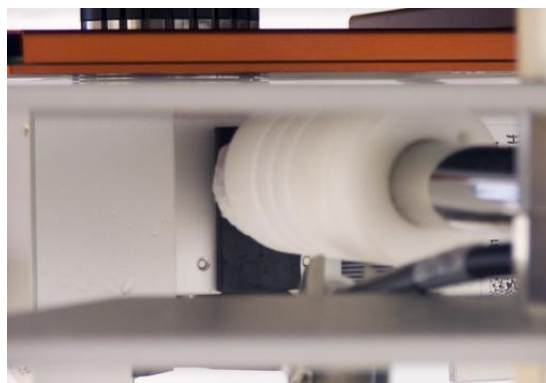
Figure 37. The cooling pipe connected to the probe of the 500 MHz spectrometer
