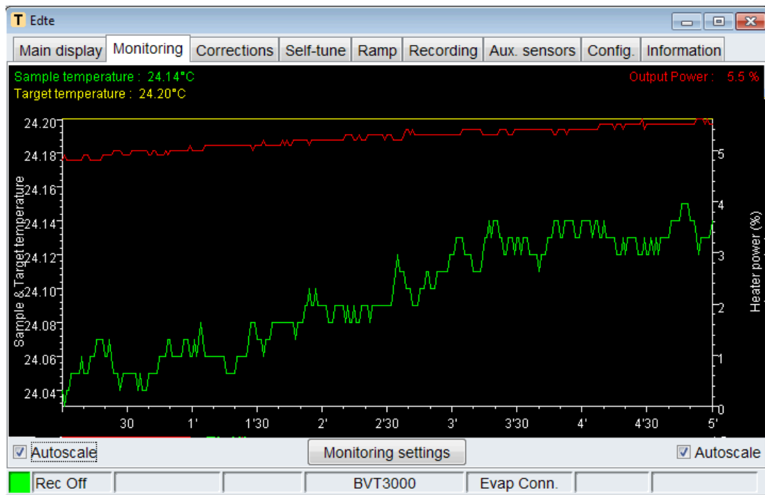
Figure 22. The edte window under the Monitoring tab for checking temperature stability
