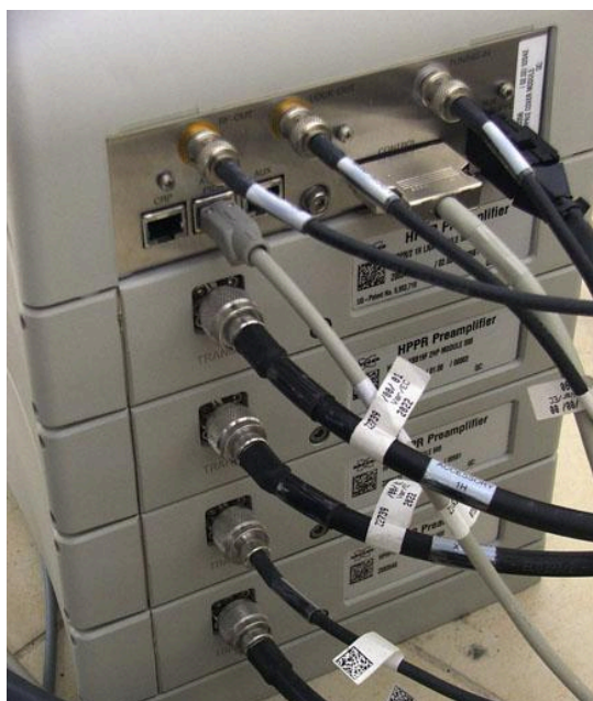
Figure 11. Connections entering the preamplifiers from the back for regular acquisition.
