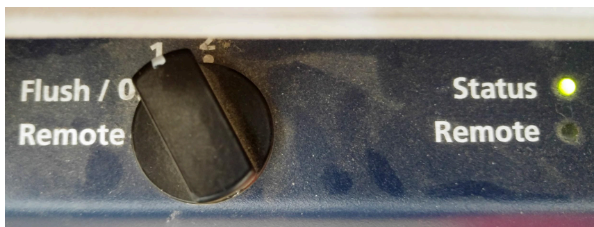
Figure 9. BCU1 top-front panel at the routine setting, mode 1, with status light green
