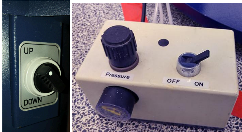
Figure 6. Switches for raising the magnet (on the floor - right and on a magnet leg - left)
