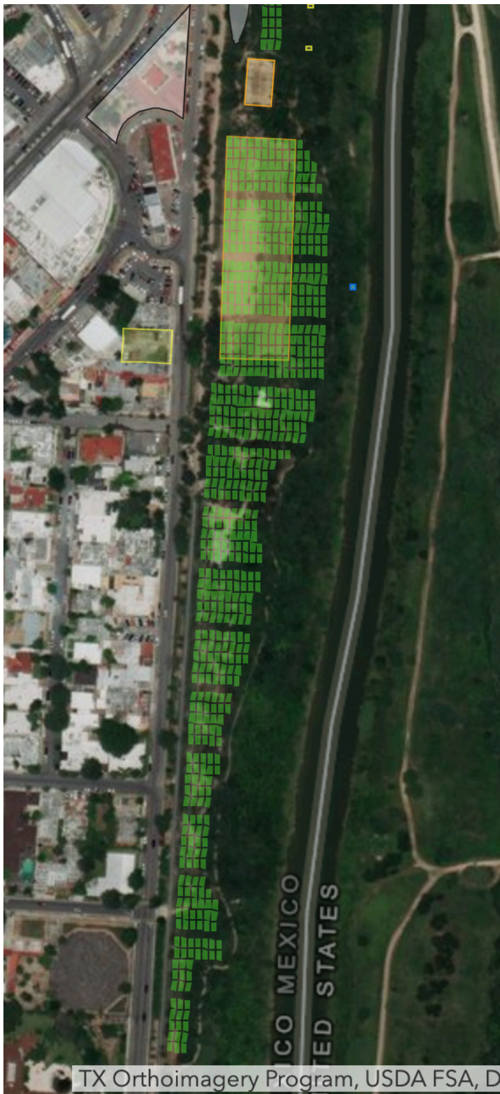
Figure 3: Satellite photo of Jardin area of Matamoros with green boxes showing a draft layout of the Better Shelter units on location. This design was prepared by the Civil Engineer department of Villanova University in Philadelphia, Pennsylvania based on available satellite imagery.
