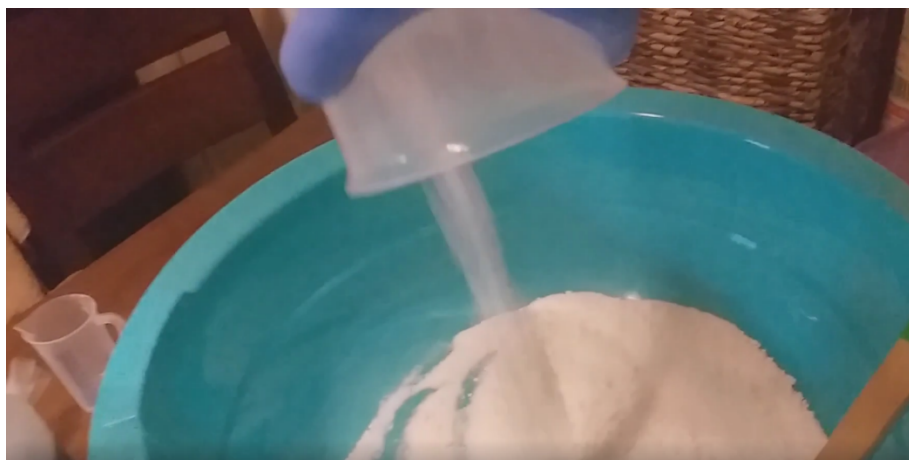
Figure 26. Foam stabilizer addition and mixing
