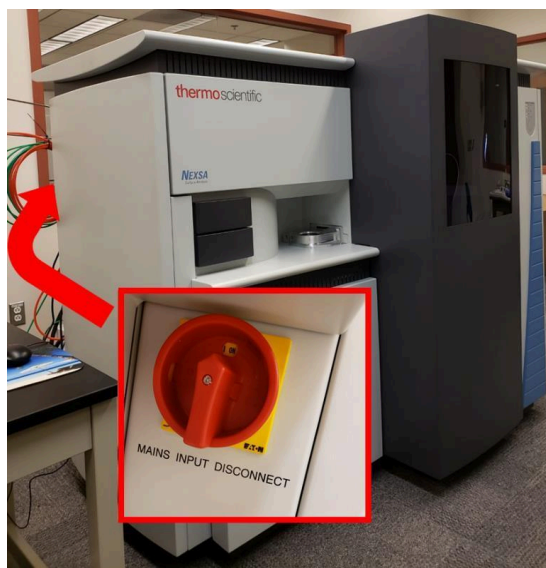
Figure 1: Picture of the NEXSA. The red arrow is pointing to the back left of the instrument, where the emergency power shut down knob is located. Turn the knob to the "off" position.
