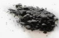
Our CR 700 series powder is insoluble in water, and odorless. It has high electrical conductivity and helps in increasing emission current. It is used in the following applications: ceramic raw material, production of semiconductor thin film, glass coating, sputtering targets, in plastics, and aerospace.
